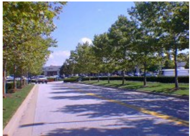
The shade from large trees reduces the amount of heat absorbed and re-radiated from paved surfaces, providing a cooling effect in summer.
